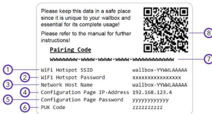
Figure 1: Descriptive illustration of the individual Configuration Sticker for each Elli Charger Connect and Elli Charger Pro
